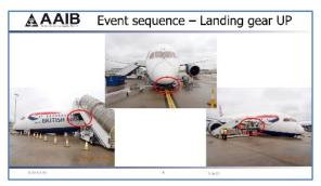
Steve described an AAIB investigation in June 2021, during Covid restrictions, where the nose landing gear of a British Airways 787-9 was inadvertently retracted on the ground. This occurred during ground maintenance operations while preparing for a cargo flight and centred on the mistaken insertion of a landing gear downlock pin into the Apex pin bore hole on the NLG mechanism, rather than the correct downlock pin hole nearby.
