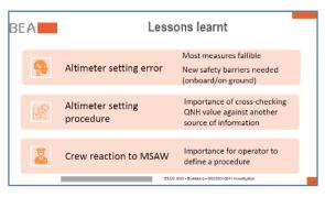
The BEA concluded there were lessons in the altimeter setting check procedure and the flight crew MSAW procedure that should be defined at the operator level. Safety Recommendations have been made to the Air Navigation Service Provider, to EASA and to ICAO to solve inconsistencies in MSAW phraseology, adding the notion of urgency to response and on the systematic recall of QNH settings.
